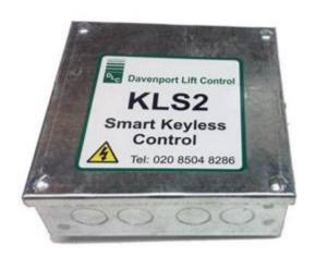
The purpose of this stylish standalone unit is to improve security in public buildings were restricted access is required. This unit can be used to isolate the lift push buttons simply by holding a programmed fob or card over the reader and the volt free contact will close for the time period programmed. This would be typically 3 seconds.
