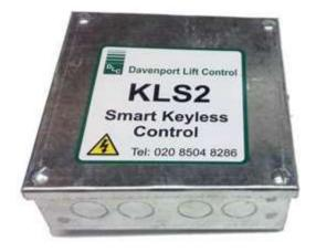
The purpose of this stylish standalone unit is to improve security in public buildings were restricted access is required. This unit can be used to isolate the lift push buttons simply by holding a programmed fob or card over the reader and the volt free contact will close for the time period programmed. This would be typically 3 seconds.
