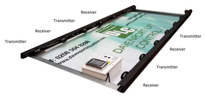
The Anti Surf Device comes in a standard-length of 1900 mm. Because all lift cars are different the unit may need to be cut down in length. The transmitters and receivers can be removed in pairs. It is important when adjusting the sensors, the minimum distance between them must be no less than 150mm. After all the sensors have been adjusted cut the lid and fit between sensors
